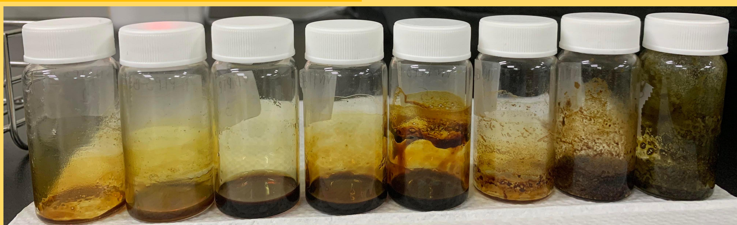
Figure 3. Eight fractions after performing reverse phase chromatography
