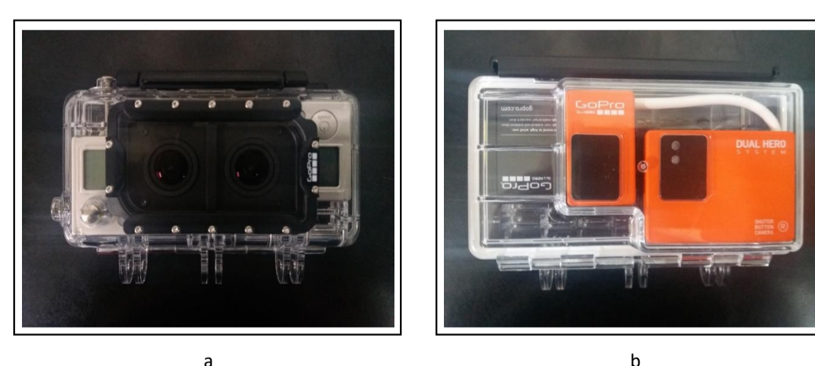
Fig 2. Two GoPro Hero 3+ embedded in a dual system dive housing (a) front view and (b) back view
